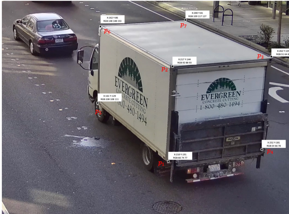
Figure 5-5 Identify seven points and obtain their pixels number for calibration
