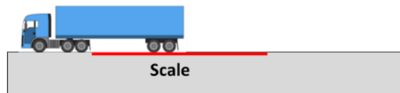
Figure 41a: Calibration Truck Weighing Procedure (Wc)
