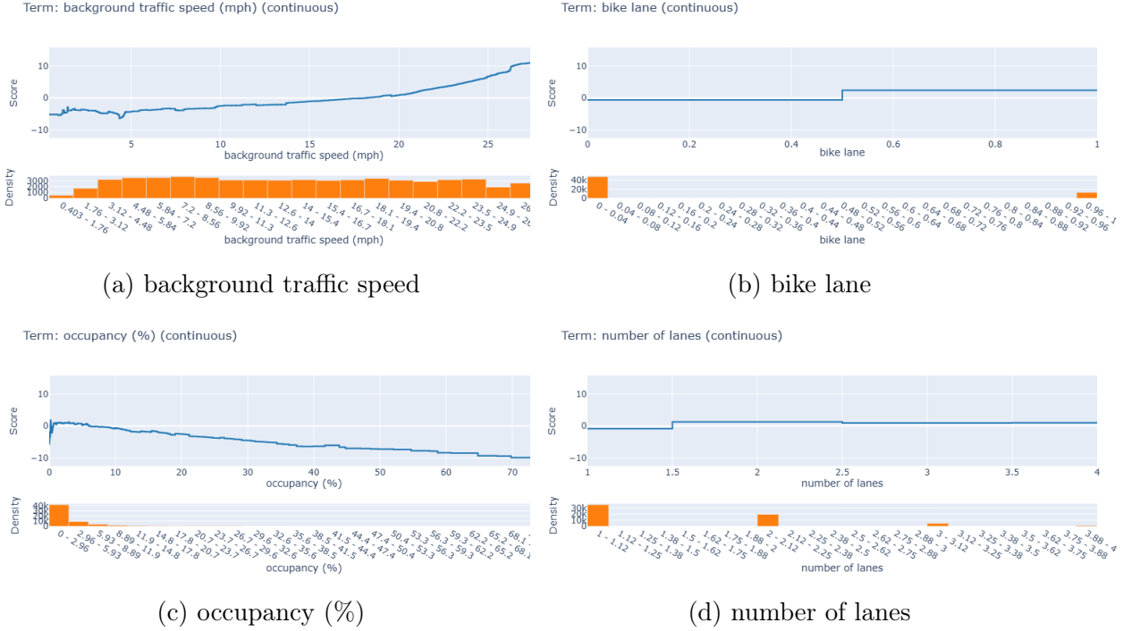
Figure 8: EMVAID shape functions for (a) background traffic speed; (b) bike lane; (c) occupancy; (d) number of lanes.
