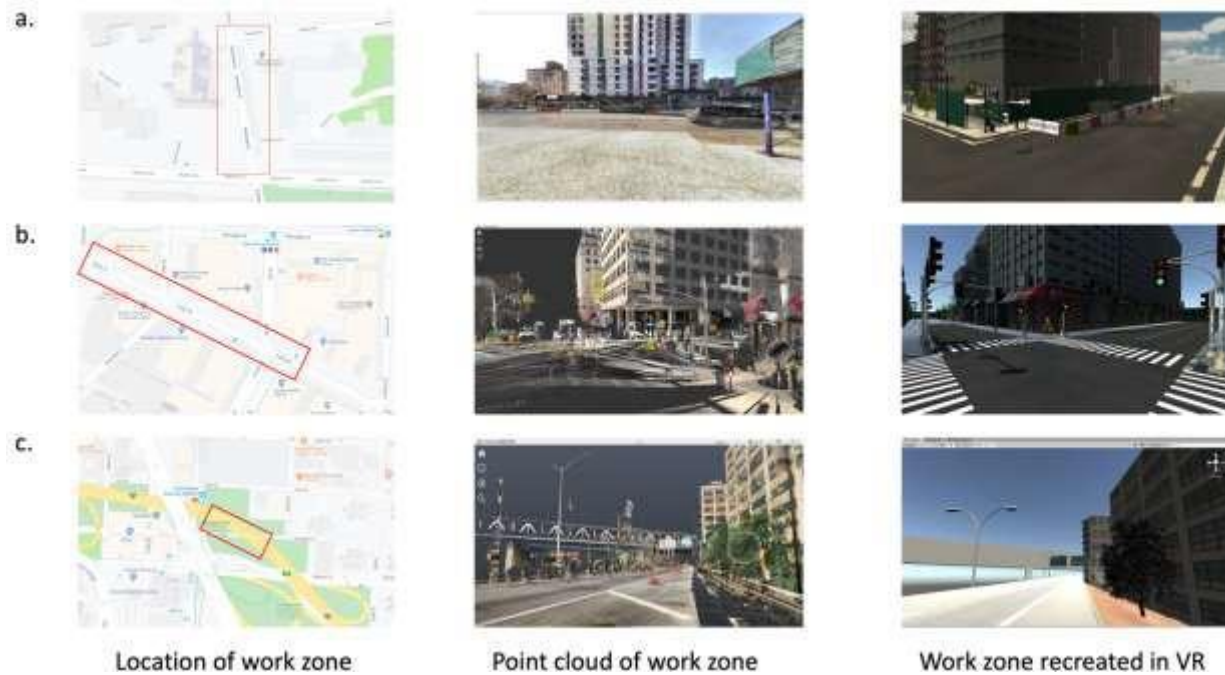
Figure 16 Three testbed scenarios captured in point cloud then converted to VR environments.
